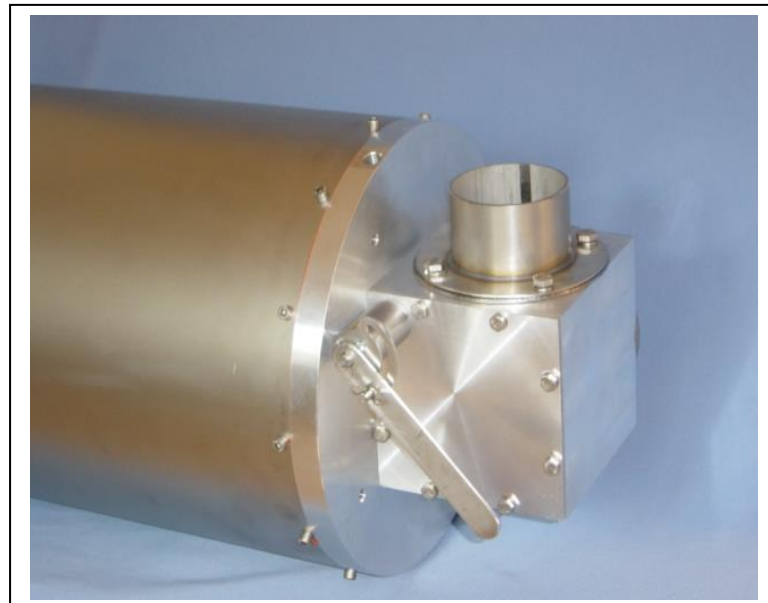
Mounted manually-controlled valve
